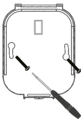
Insert fixing screws through mounting holes of the power base and tighten.
